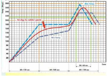
Fig 2. Infrared soldering profile
