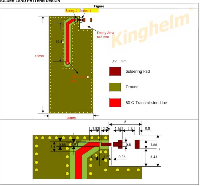
Antenna on Test Board (Thickness 1.2mm)
