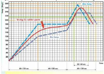
Fig 2. Infrared soldering profile
