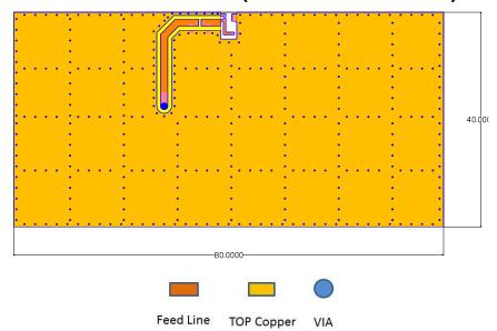
2<sup>nd</sup> Evaluation Board Dimension Evaluation Board Dimension (board size 80x40mm)
